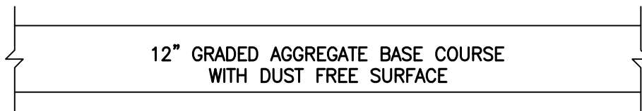
ALTERNATE - GRAVEL SURFACE SECTION
